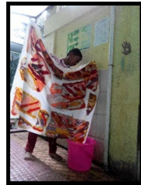
Figure 11 Dyeing by dipping
